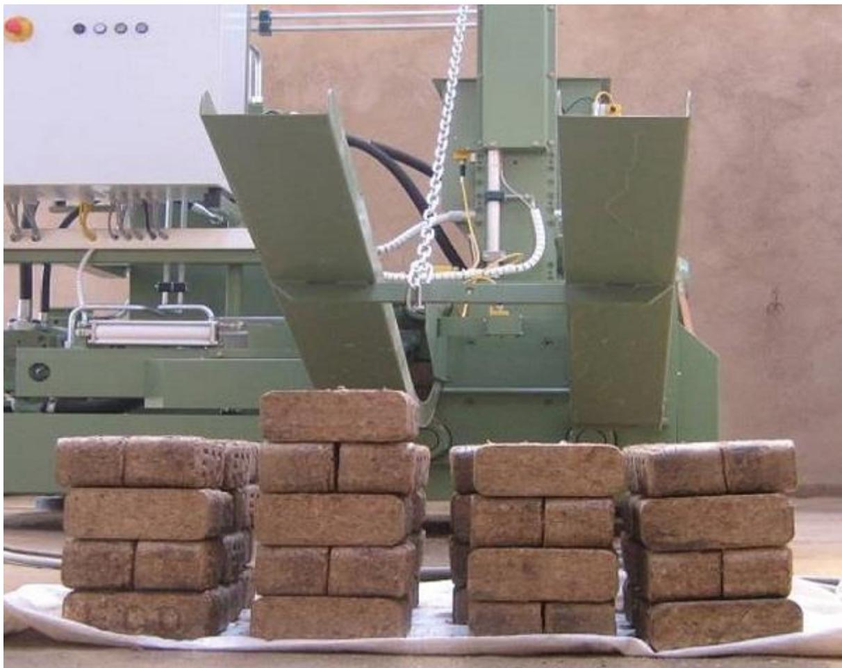
Briquette production operations at Kigali-based COPED Ltd. The products serve as a substitute to wood and charcoal for cooking. PHOTO | COURTESY
