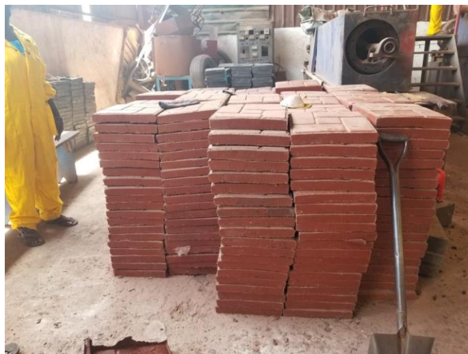
Samples of bricks produced from plastic waste at the Nelplast manufacturing plant in Accra – Ghana. Zubaida Mabuno Ismail.
